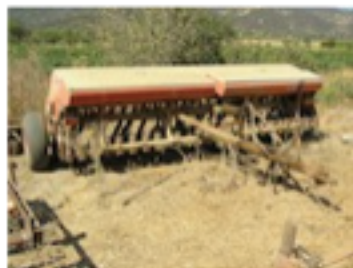
A grain drill. Separate seed boxes allow seeding of a grain and legume at the same time.
