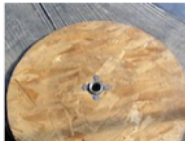
The plywood round for a drip winder. The threads of a flange are showing through the center. T nuts hold the flange in place.
