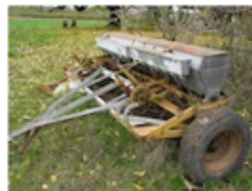
A grain drill. Separate seed boxes allow seeding of a grain and legume at the same time.
