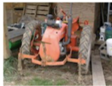
Rear tool bar on G with sweeps set up behind wheels. The center sweep is in its storage position. Sauvie Island Organics, Portland, OR
