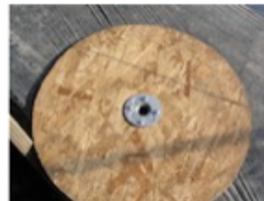
The flip side of the plywood round with a flange mounted at the center.
