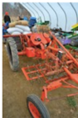
A farm built Lely tine weeder for the G. Hearty Roots Farm, Tivoli, NY
