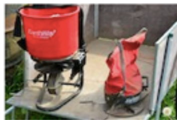
The plastic hopper type broadcast spreader on the left holds about 2 times the amount of seed as the bag type spreader on the right but basically functions the same way. It also has larger gears that will last longer than the bag type.
