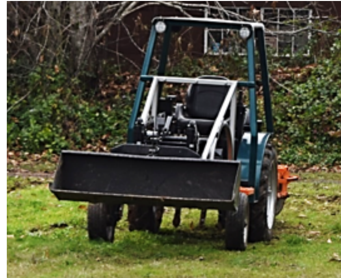
Prototype #2: DC motor; Lithium batteries; used transmission; front, mid & rear hitch
