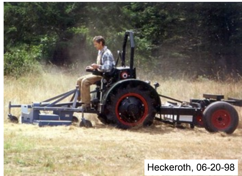
Scratch-built with wheel motors, adjustable seat and solar shade canopy 1996 First use of linear actuators, exchangeable battery packs and remote control
