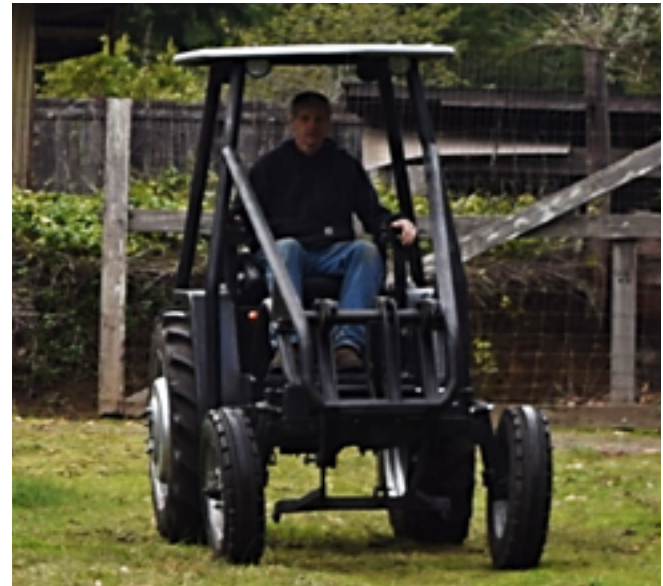
Prototype #4: AC motor; Lithium batteries; NEW transmission; HC; front, mid & rear hitch
