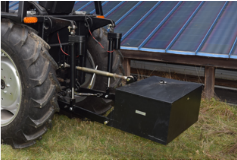
Exchangeable battery pack can be quickly mounted on any hitch for extended run time
