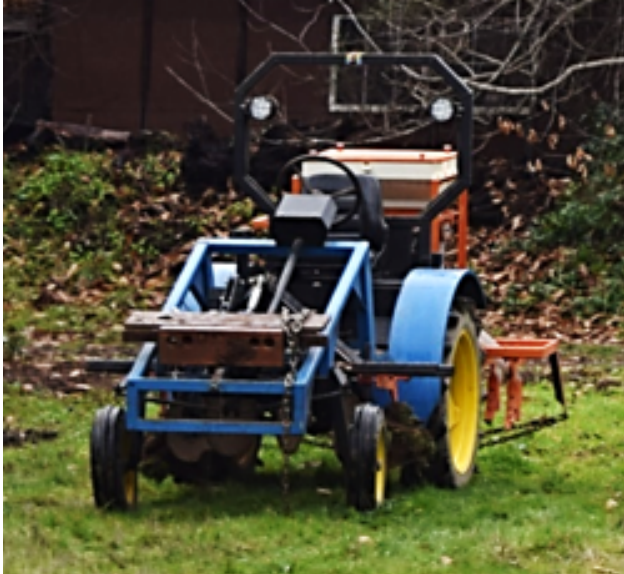
Prototype #1: AC motor; lead acid batteries; used transmission; no front hitch
