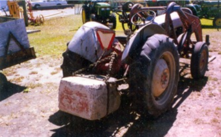
Tractors require weight for traction
