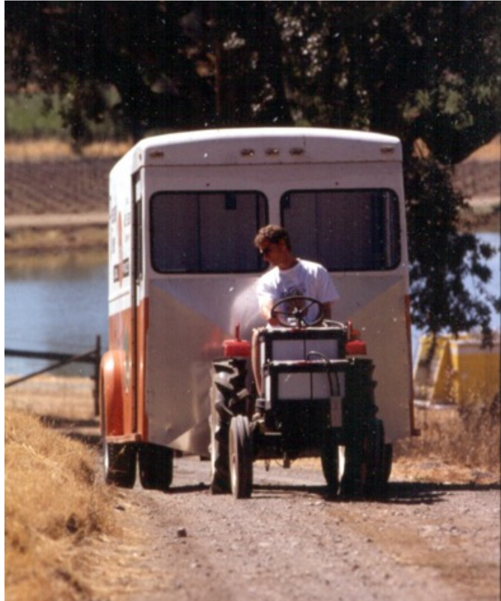
Batteries provide useful weight for traction
