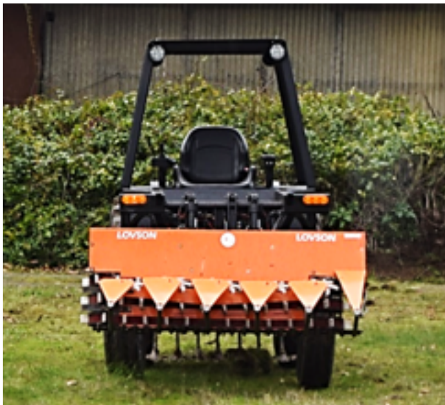
Prototype #3: AC motor; Lithium batteries; used transmission; front, mid & rear hitch
