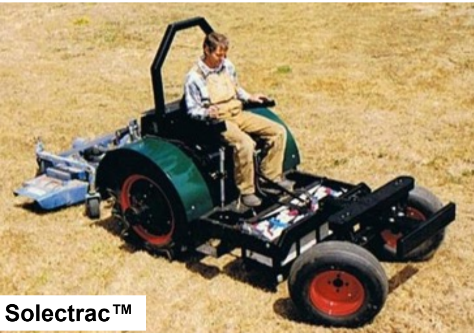
Scratch-built with wheel motors, adjustable seat and solar shade canopy 1996 First use of linear actuators, exchangeable battery packs and remote control
