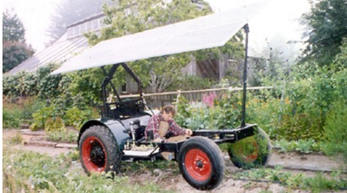
Scratch-built with wheel motors, adjustable seat and solar shade canopy 1996 First use of linear actuators, exchangeable battery packs and remote control
