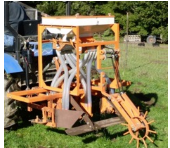
Rear hitch with PTO can carry and power any Category 1 implement
