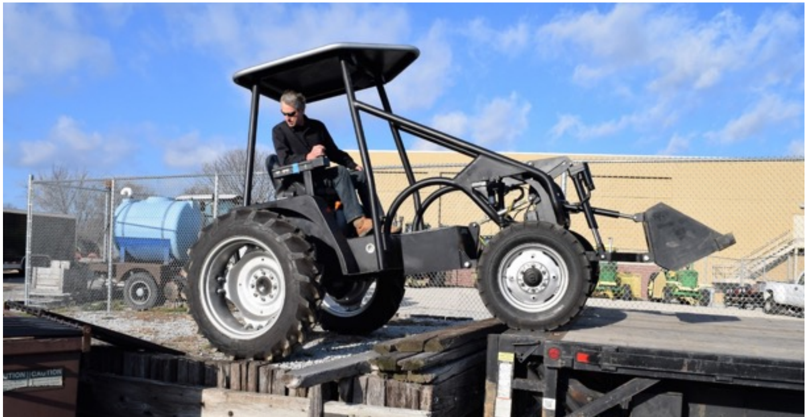
Unloading the eFarmer at the International Testing Lab with the exchangeable pack on the mid hitch and loader bucket on the front hitch
