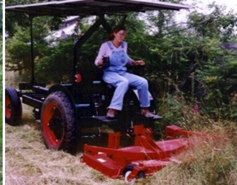
Scratch-built with wheel motors, adjustable seat and solar shade canopy 1996 First use of linear actuators, exchangeable battery packs and remote control
